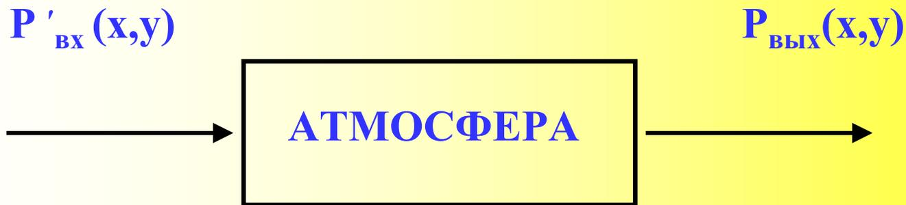
$$P_{ВЫХ}(x,y) = P'_{ВХ}(x,y) ** h_g(x,y)$$
