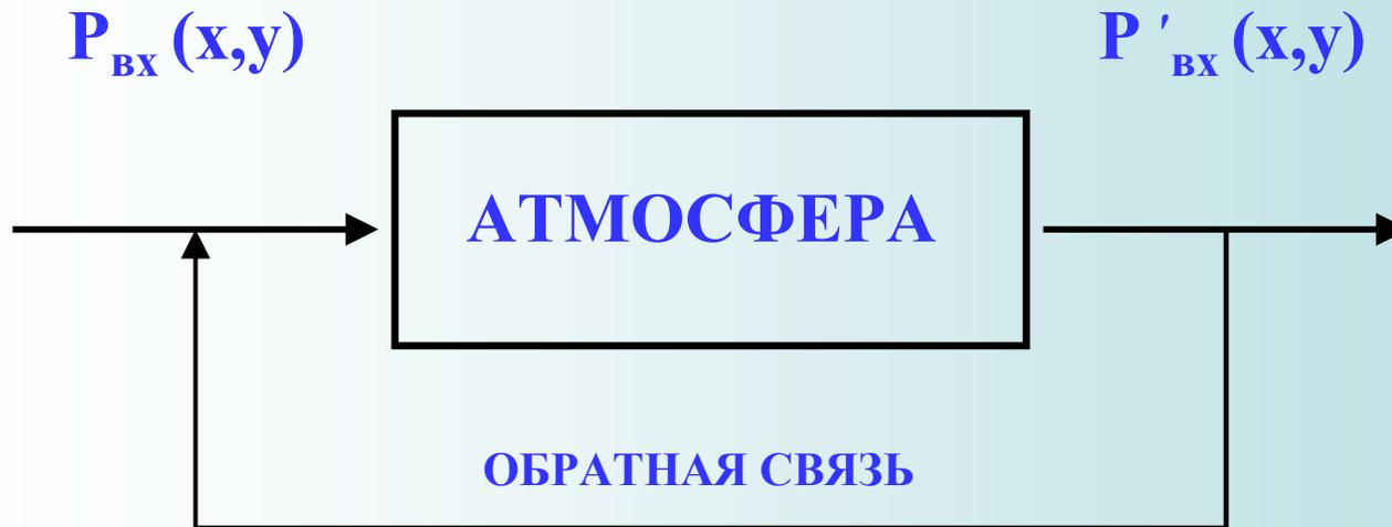
$$P'_{ВХ}(x,y) = P_{ВХ}(x,y) ** h_{gg}(x,y)$$
