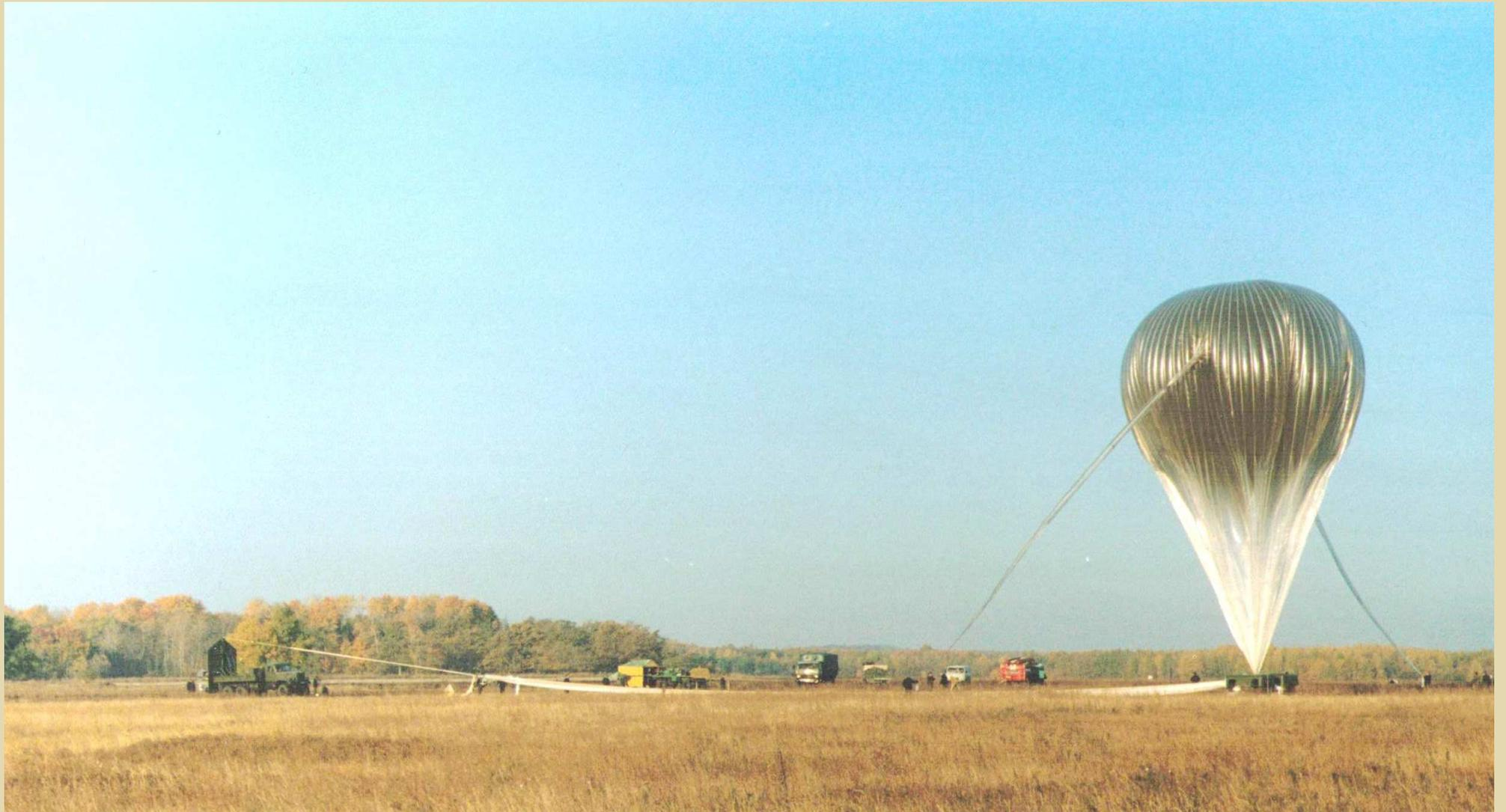
**Balloon magnetic gradiometer at the starting position
